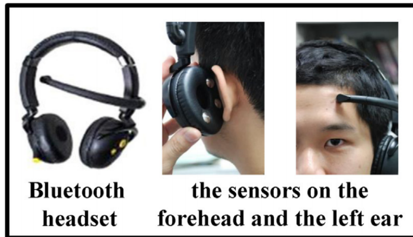
Figure 3.12: Neurosky headset - Three Sensors on the left ear and the fourth on the forehead leftside Yang et al. [32]
